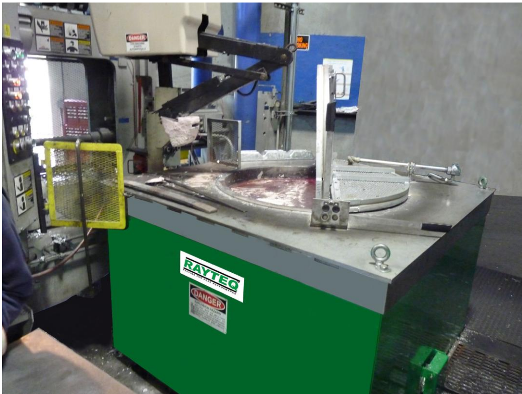
RAYTEQ MODEL DC-720 HAS BEEN MELTING RIGHT AT A DIE CASTING MACHINE TWO SHIFTS PER DAY, FIVE DAYS PER WEEK SINCE JUNE, 2009 WITH ALL ORIGINAL RAYTEQ HIGH-POWER HEATING ELEMENTS STILL IN OPERATION. PHOTO COURTESY OF A & B DIE CASTING, HERCULES, CALIFORNIA.
