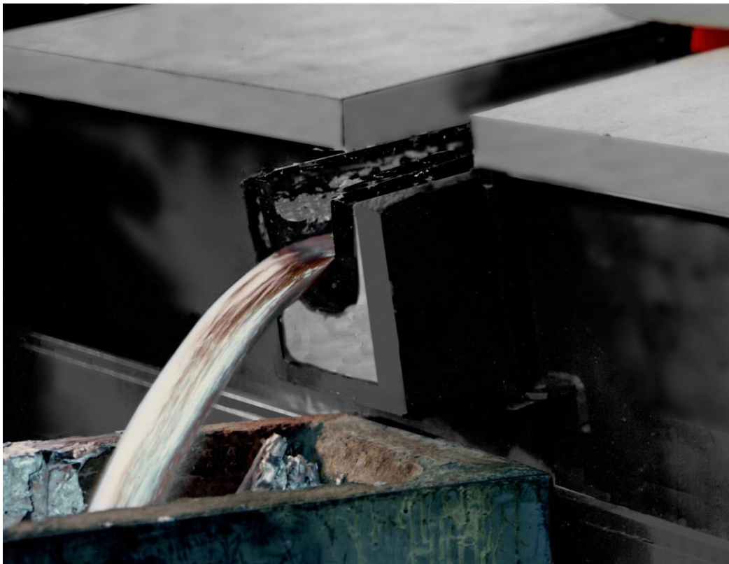
MOLTEN METAL STREAM FROM TILTING CRUCIBLE-TYPE ALUMINUM MELTING FURNACE HAS INCREASED SURFACE AREA WHICH REACTS WITH WATER VAPOR AND OXYGEN TO FORM DROSS AND HYDROGEN POROSITY, MAJOR CONTRIBUTORS TO CASTING DEFECTS.
