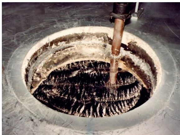
CLEAN MOLTEN ALUMINUM BATH SURFACE WITH ELECTRIC RESISTANCE MELTING
