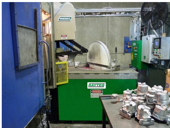
RAYTEQ ELECTRIC FURNACE MELTING RIGHT NEXT TO 950 TON BUHLER-PRINCE DIE CASTING MACHINE
