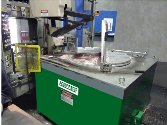
MELTING RIGHT AT THE DIE CASTING MACHINE WITH RAYTEQ ELECTRIC ALUMINUM MELTING FURNACE
